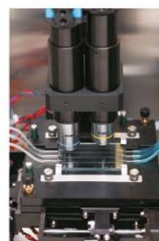
Faster sampling and analysis with 3 flow cells to hold samples, duo lens and duo cameras for quicker analysis and better results.
